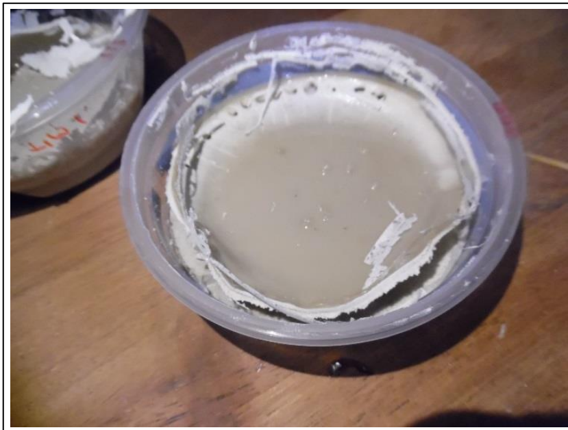
Fig. 3: Excessive shrinkage from the 100:55 quartz flour : lithium silicate formulation when poured into an open impervious cup. This result led to the alternative test methods relying on more replicative applications to vertically oriented cavities.
