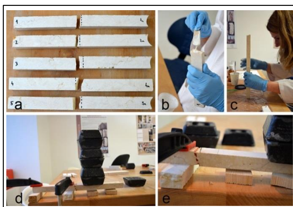
Fig. 1: Preparing samples and cantilever test: a – limestone samples; b – applying the adhesive mixture 1; c – setting of samples; d and e – cantilever test.
