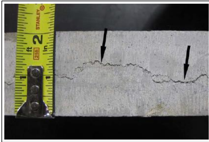
Fig. 3: Microcracks parallel to stone face.
