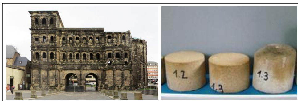
Fig. 1: The Porta Nigra in Trier and drill cores showing brown discolouration after testing for capillary water absorption.
