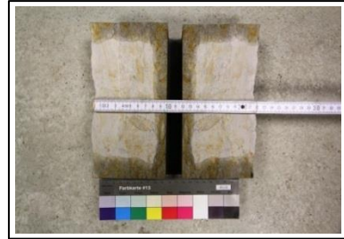
Fig. 4: Test cube penetrated by Funcosil 300E with total immersion under atmospheric pressure and cut parallel (above) and normal to bedding (below) immediately after the procedure (photos: M. Eilenberger).
