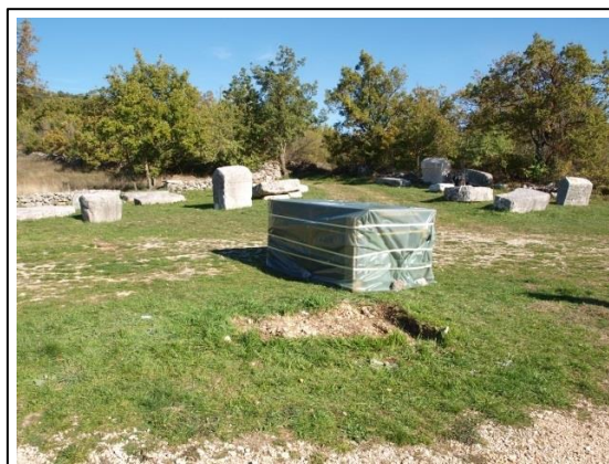
Fig. 5: The improvised pool with ammonium oxalate bath, Crljivica.
