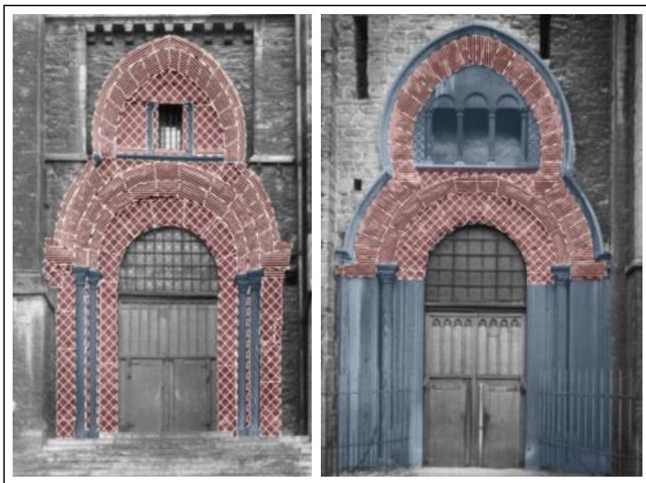
Fig. 3: Mapping of the bedding planes of the original stone blocks in the Mantile (left) and Capitole portal (right). Hatchings underlines the bedding planes, while crosshatching is used for face-bedded blocks. Blue-coloured zones correspond to the 19th century restoration with Belgian bluestone ©KIK-IRPA, Brussels.
