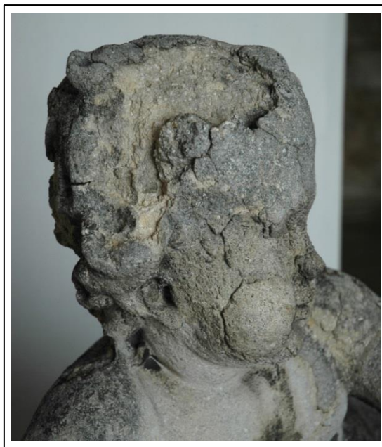
Fig. 11: Photograph of a limestone statue surface-treated with ESE 300 20 years ago.
