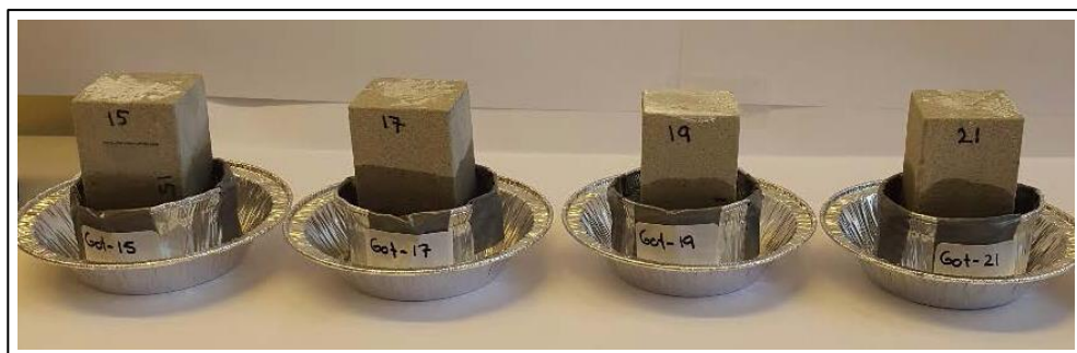
Fig. 3: Suction test after ED.
