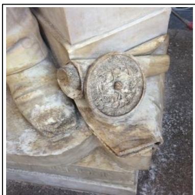
Fig. 9: Signature of Carlo Ottavio Castiglione's statue (1855) during the cleaning using sulfate-reducing bacteria applied to the surface with the aid of a gelatinous medium. The cleaning has brought to light (for example in the right area of the cartouche) some punctual spots along the surface. FTIR analysis carried out by Palladio Analisi s.r.l. laboratories identified calcium carbonate, gypsum, silicates, and very feeble traces fluorosilicate absorptions, which are most probably left by residues of protective and polishing products used in the past.
