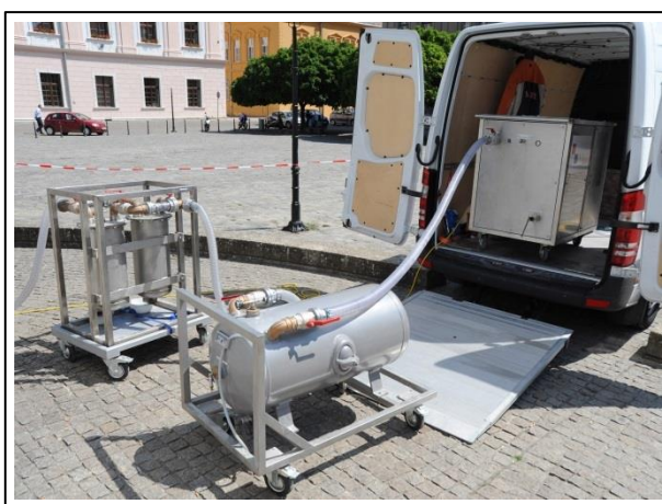
Fig. 1: Mobile VCP equipment, vacuum pump (in the back of the van), balance tank (middle), tank A&B combination (left; see Fig. 2 for further details).
