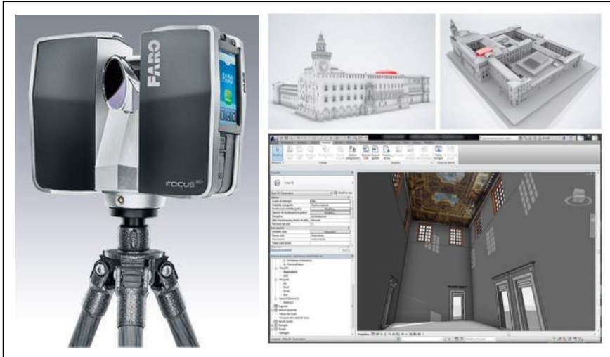
Fig. 1: 3D Laser Scanner and Historic Building Information Modelling (HBIM).
