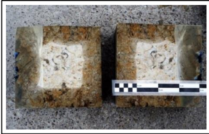
Fig. 3: Test cubes penetrated by Funcosil 300E with VCP and cut parallel to bedding immediately after the procedure (photos: E. Pummer).
